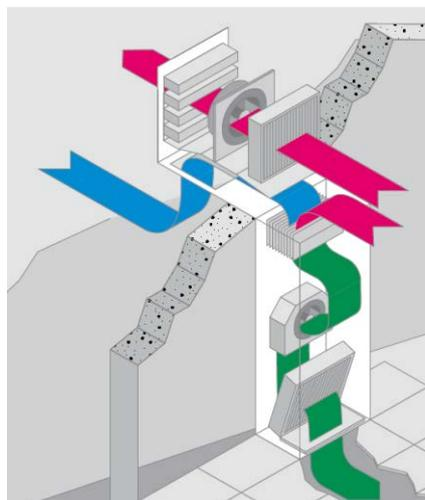
**Figure 5: Direct free cooling**
