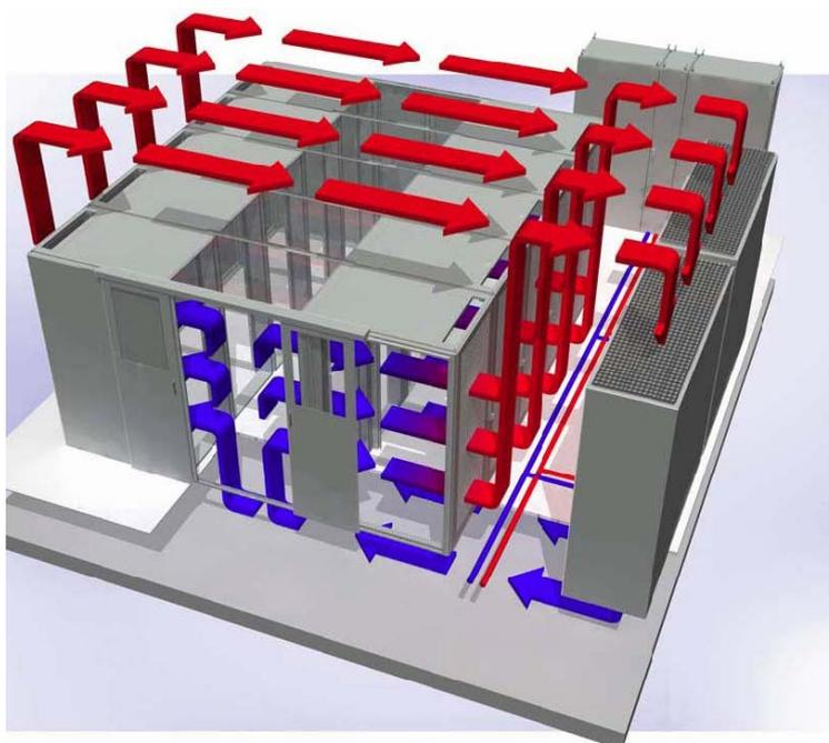
**Figure 2: Function principle of cold aisle containment**
